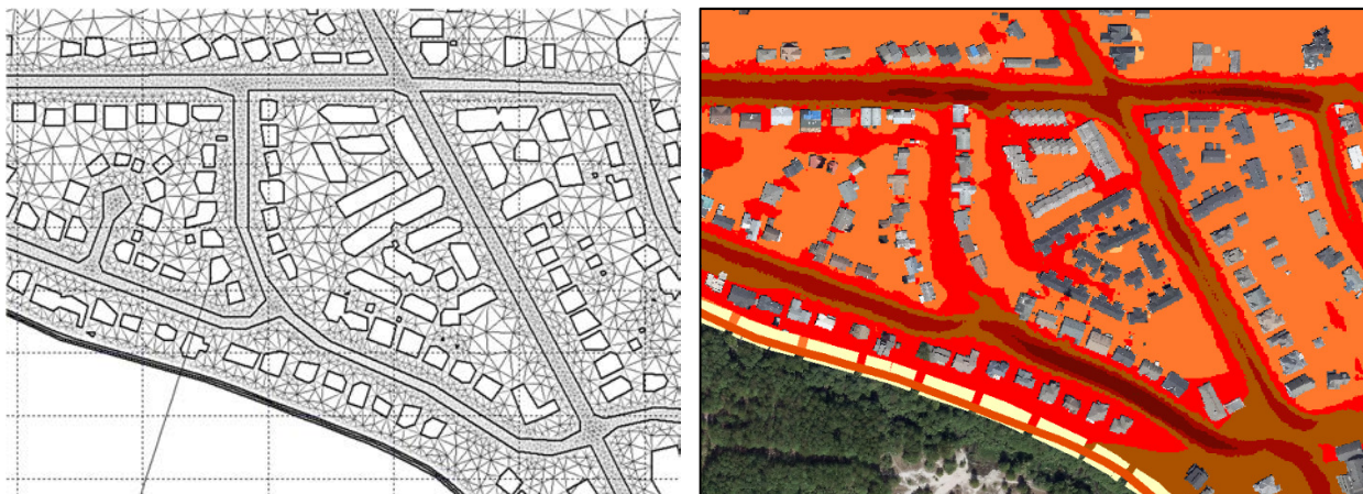
Figure 3: Detailed representation of the floodplain (left) supports a more nuanced analysis of maximum Hazard Rating (depth x velocity, right), particularly where flow is concentrated along the road network
